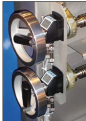
[1] Highest flexibility: The same basic device with programming adjusted to the application. [2] Easy optical upgrading via compatible mounting dimensions of mechanical and electronic position indicators. [3] Multiple format settings with AP04: Folding box production requires a number of adjustments. [4] Automated handwork: bus-compatible position indicator AP04 for controlled spindle positioning.
